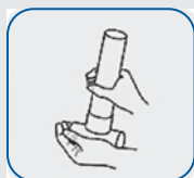
Test Dryfit of the joint
