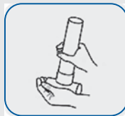
Test Dryfit of the joint
